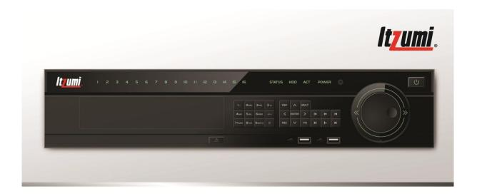
**HKIZ-16960H**: Full channel 960H recording,16 channel video inputs, 16 channel audio inputs, 16 channel loop outputs and 1 channel spot output with multi split display. It can support HDMI, VGA, eSATA, USB2.0 and 8 HDDs.
