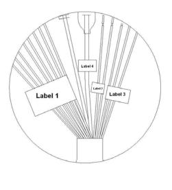
Label 1 Purple: ALARM\_COM Brown: ALARM\_OUT Red: ALARM\_IN1 Orange: ALARM\_IN2 Yellow: AUDIO OUT Black: GND Green: AUDIO GND White: AUDIO IN
